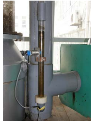
Magnetic induction Water Level Meter
