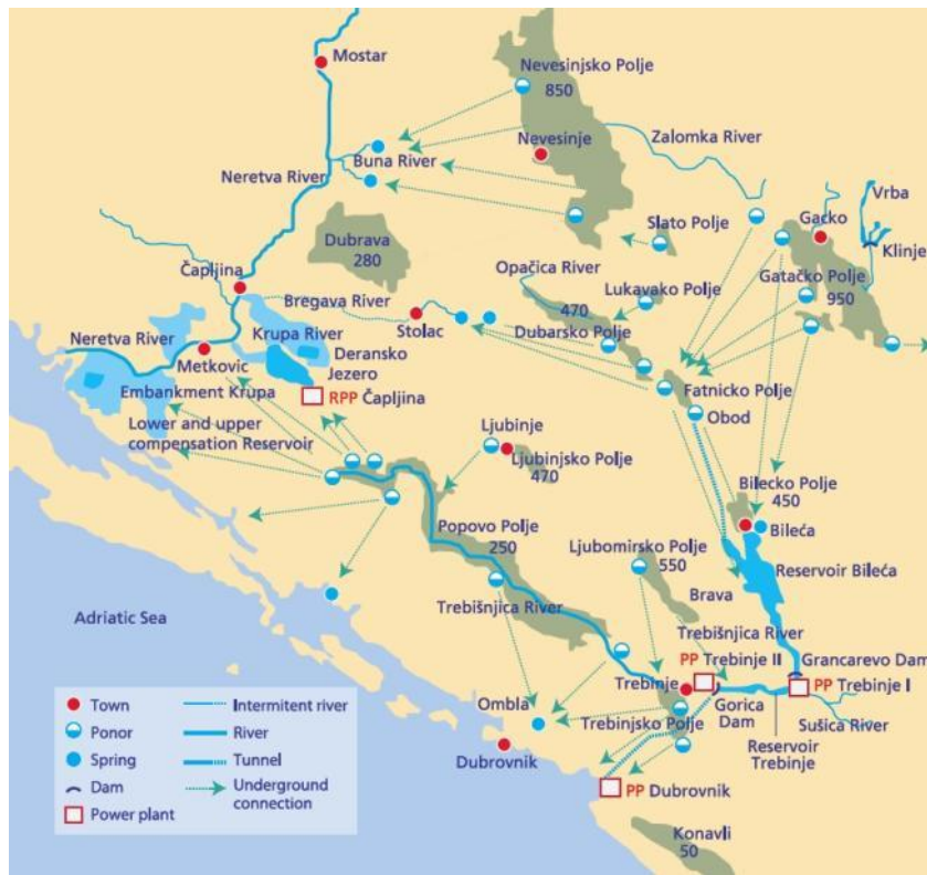
Figure 3.25 Connections between ponors and springs in the East Herzegovina region confirmed by dye tests
