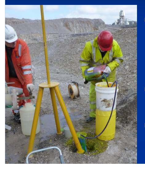
10330 g of 40% sodium fluorescein (uranine) was diluted with ~450 L of water over a 30 minute period and injected below the standing water level using a siphon system and a hosepipe.
