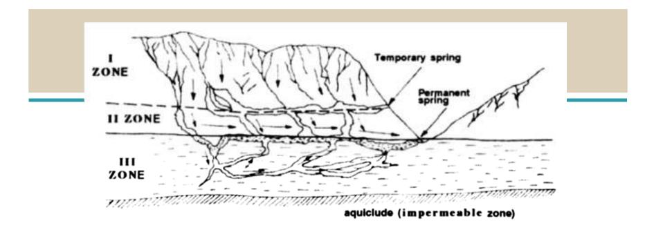
Figure 3. - Schematic hydrogeological cross-section of the karstic aquifer which lies on the aquilude substratum; the superposition hidrogeologic zones (after Cvijic hypothesis)
