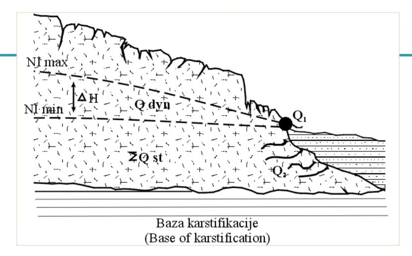
• Natural groundwater reserves of karst aquifer – dynamic & static (case with ascending spring Q1 and underground discharge Q2)
