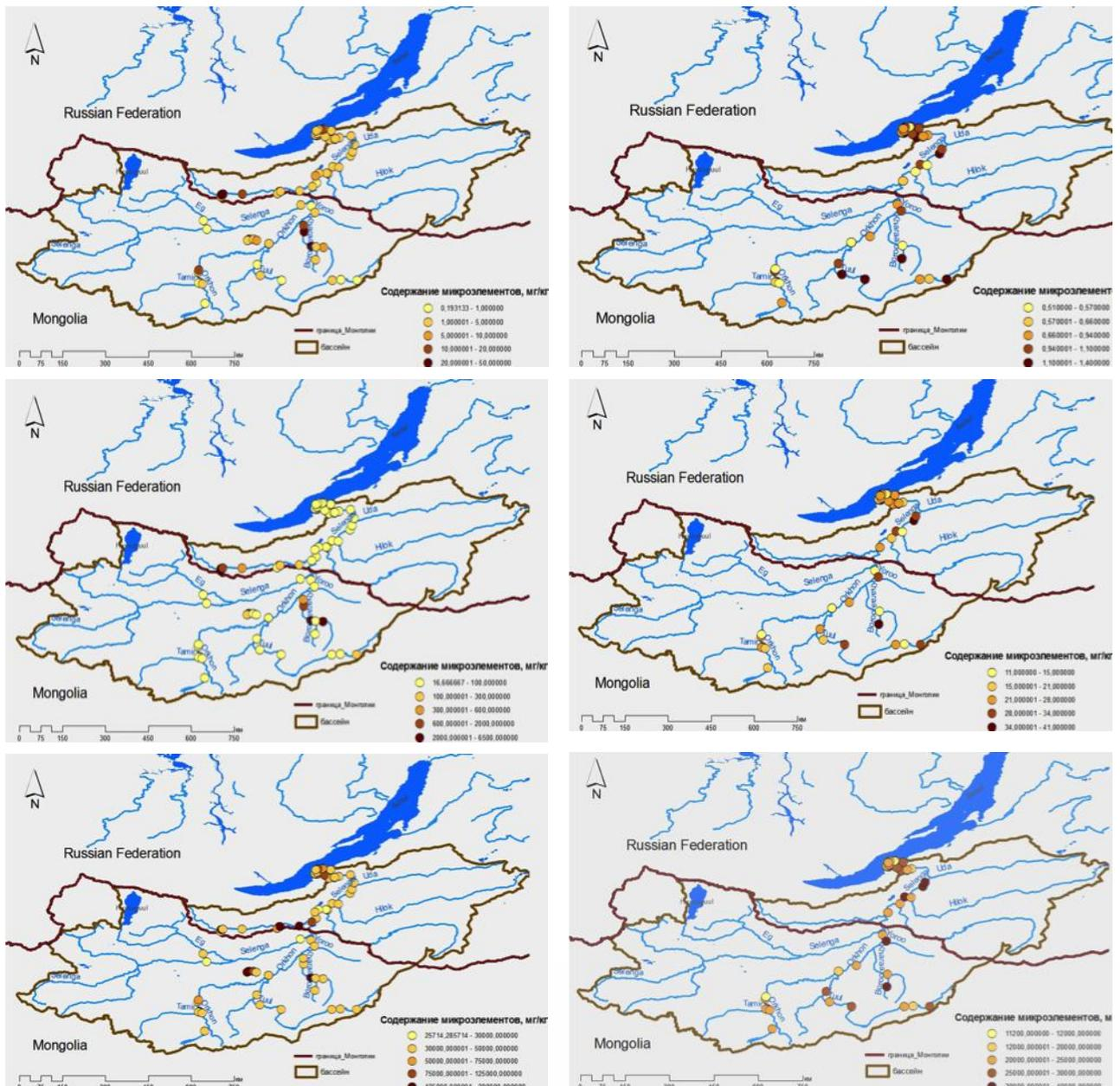
**Figure 4.4.2.a** Concentration of heavy metals in suspended sediments in the Selenga River Basin between July-Aug 2011. From left to right, top to bottom: molybdenum, copper, and iron (mg/kg).
