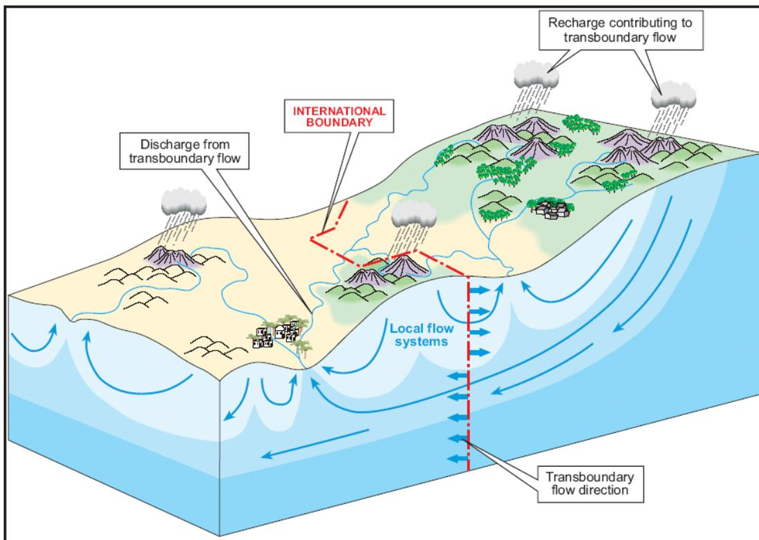
**Figure 4.3.1** Simplified diagram demonstrating the transboundary relationship between upstream and downstream surface and groundwater flow systems (UNESCO 2002).
