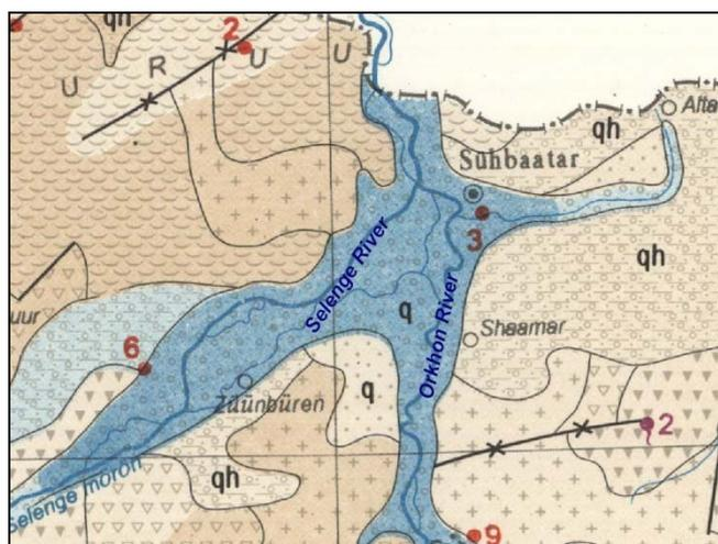
**Figure 2.5.** Confluence of the River Selenga and River Orkhon (q: fluvial deposits of Quaternary age, qh: fluvial deposits of Holocene age, qp: fluvial-lacustrine deposits of Pleistocene age, map scale 1 000 000 (Jadambaa, N., Enkhkhishig, 1996)
