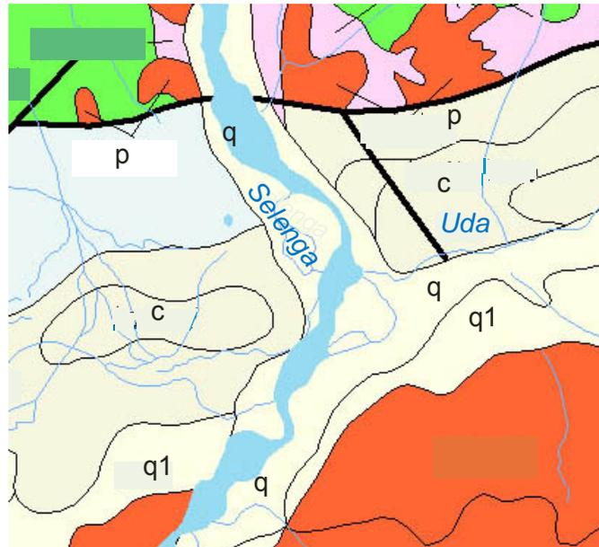
**Figure 2.7.** Confluence area of the River Selenga and River Uda, (q: fluvial deposits of Holocene age, q1:luvial deposits of Quaternary age, c: fluvial deposits of the Cretaceous age, p: metamorphic-volcanic and metamorphic sedimentary rocks of Paleozoic age), scale 1: 200 000 (Yalovik, 2007)
