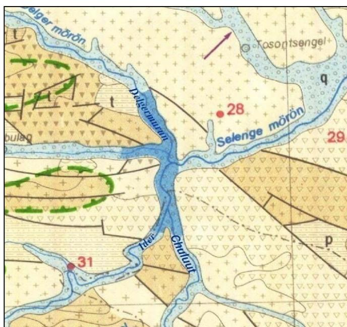
**Figure 2.1.** Confluence area of the Rivers Delgermurun, Ider and Chuluut (q: fluvial deposits of Quaternary age, t: sedimentary rocks of Triassic age, p: intrusive and volcanic rocks of Permian age), map scale 1 000 000 (Jadambaa, N., Enkhkhishig, 1996)
