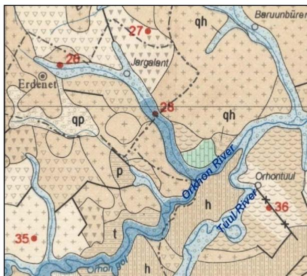
**Figure 2.3.** Confluence area of the River Orkhon and River Tuul (qh: fluvial deposits of Holocene age, qp- lacustrine deposits and carbonate rocks of Pleistocene age, t: sedimentary rocks of Triassic age, h: meta-sedimentary rocks of Carboniferous age, p: sedimentary rocks of Permian age), map scale 1 000 000 (Jadambaa, N., Enkhkhishig, 1996)
