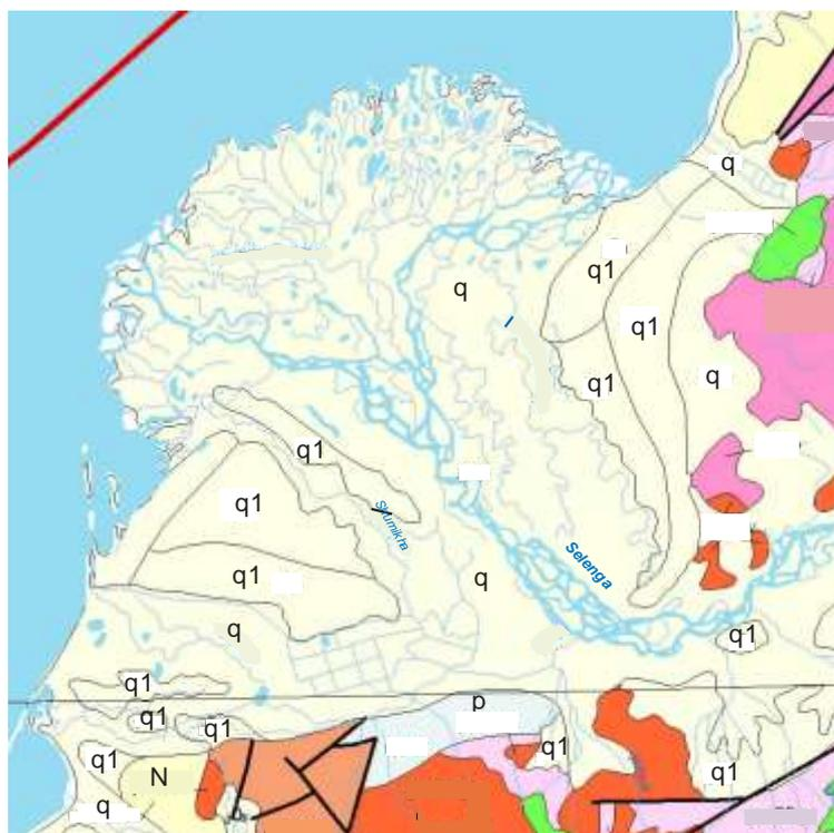
**Figure 2.9.** Delta of the River Selenga (q: fluvial deposits of Holocene age, q1: fluvial deposits of Quaternary age, N: fluvial deposits of Neogene age, deposits of Jurassic age), scale 1: 500 000 (Yalovik, 2007).
