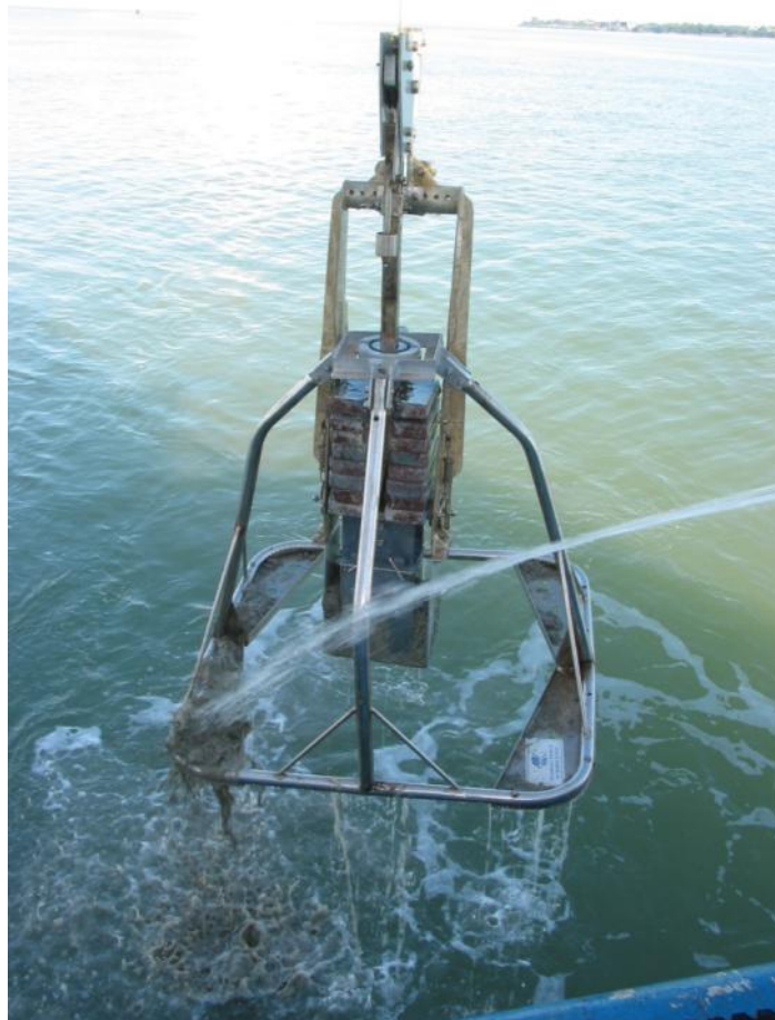
Photo 20 Bouma box corer with sediment sample.
