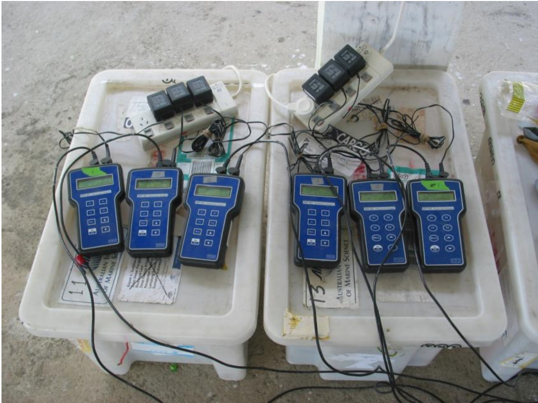
Photo 11 Oxygen meters for benthic flux measurements.
