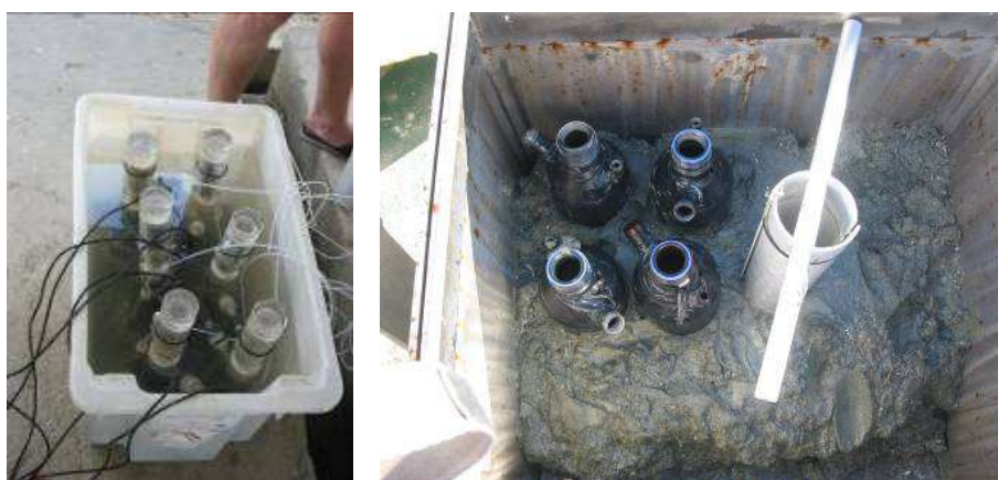
Figure 8.2. Opaque chambers for measuring dissolved oxygen
